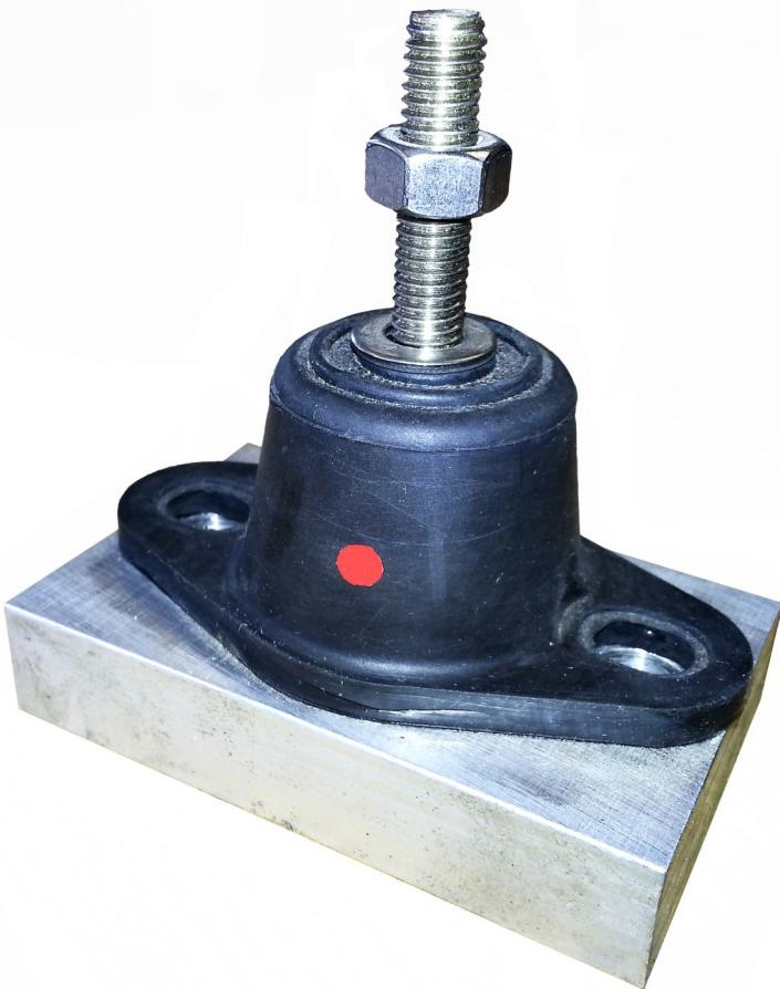
Marine Rubber Turret mountings are designed to provide superior attenuation of medium to high frequency vibration and noise emanating from a wide range of motor driven machines particularly axial and centrifugal fans.
