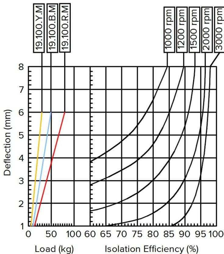
Isolation efficiency is based on dynamic rather than static stiffness for accurate calculation of system performance.
