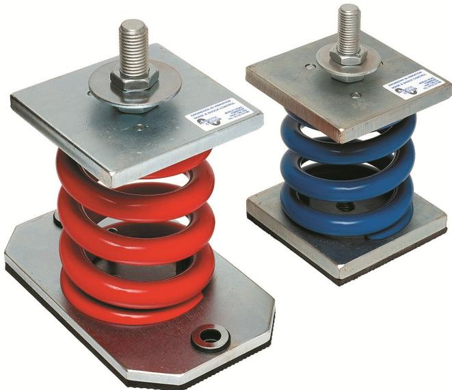
Originally designed for use with Type IPF Inertia Pouring Frames, the OS Mountings are now widely used to isolate vibration from every conceivable type of rotating and reciprocating machine. Where control of transient motion is required Open Spring Mountings can be used in conjunction with our Viscous Dampers Type SFD.
