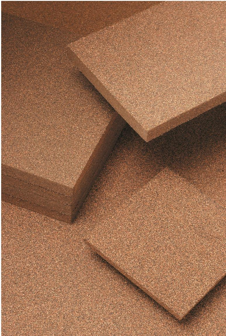
Neoprene Bonded Cork (NBC) pads are a simple solution to the problem of high frequency noise and vibration produced by many industrial machines.
