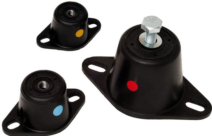
Type RM Rubber Turret mountings are designed to provide superior attenuation of medium to high frequency vibration and noise emanating from a wide range of motor driven machines particularly axial and centrifugal fans.
