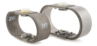
Type XM shock mountings are highly effective in reducing the transmission of vibration, structure-borne noise and shock from a wide range of rotating and reciprocating machinery. Also in protecting sensitive apparatus from external disturbances. They are specifically designed to replace the X mounting in higher ambient temperature environments.
