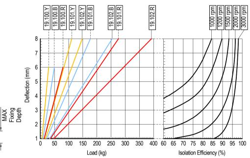
Isolation efficiency is based on dynamic rather than static stiffness for accurate calculation of system performance.
