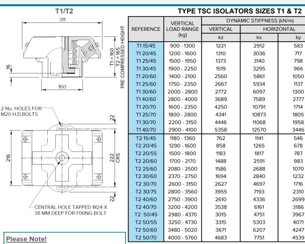
All values of stiffness are nominal subject to ±15% variation on final assembly. The isolator rubber elements are pre-loaded 6 mm upon assembly.
