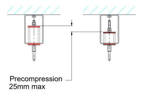
10) Ensure hangers are not over loaded when installed. Check springs are not coil bound or elements deflected more than limits allowed in our leaflets.
