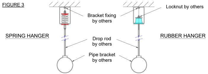
7) Depending on the amount of hanger element deflection, either by design or as required by specification, (see our appropriate leaflets) drop rods will require adjustment. This should be done on spring hangers by slackening top locknuts on drop rod inside hanger and then adjusting lower nut until correct height of pipe work requirement is achieved.
