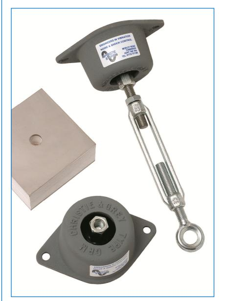
Image above shows 100 x 100 square Monolux a CRM2 Hanger with M12 turnbuckle/eyebolt and CRM2 Mounting with M12 fixings for the equipment.
